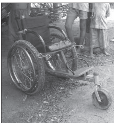
Figure 9.74. Mekong wheelchair with foot-rest, also used as a transfer-seat.
