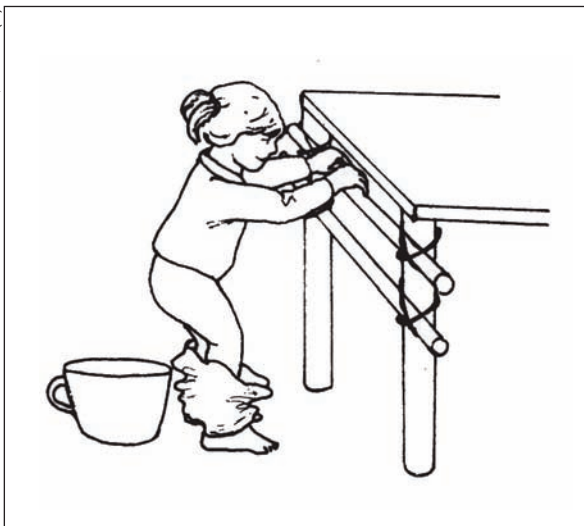
Figure 7.10. 'Ladder' of rails to help a child pull herself up and lower herself down.
