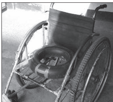
Figure 9.20. Tyre inner tube in place.
