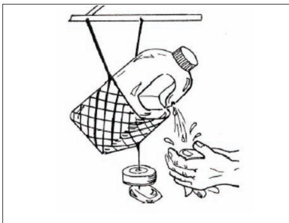
Figure 6.40. Tippy tap for handwashing.
