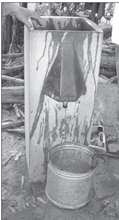
Figure 9.59. Sand water filter.
