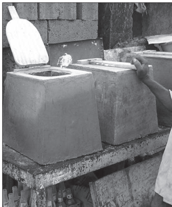
Figure 7.27. Concrete toilet seats on sale, with hinged wooden lid to reduce flies and smells.
