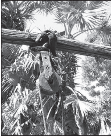
Figure 9.52. Locally made wood and metal pulley.
