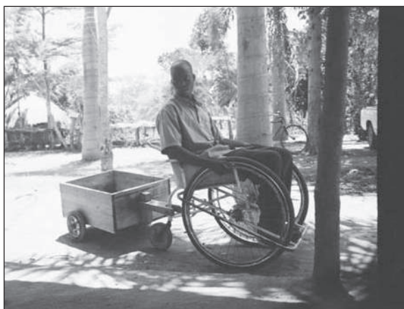
Figure 6.29. Two-wheeled wooden wheelchair trailer.
