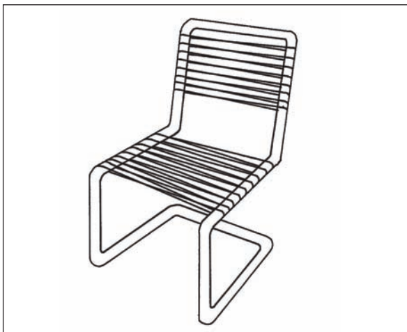
Figure 6.54. Steel tube frame bathing chair with seat and back of woven plastic strips.
