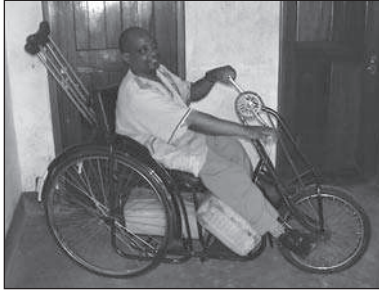
Figure 9.111. Two jerry-cans under the seat of Kiyaga's old wheelchair.
