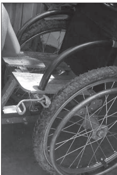
Figure 9.75. Wheelchair seat with central plank removed.
