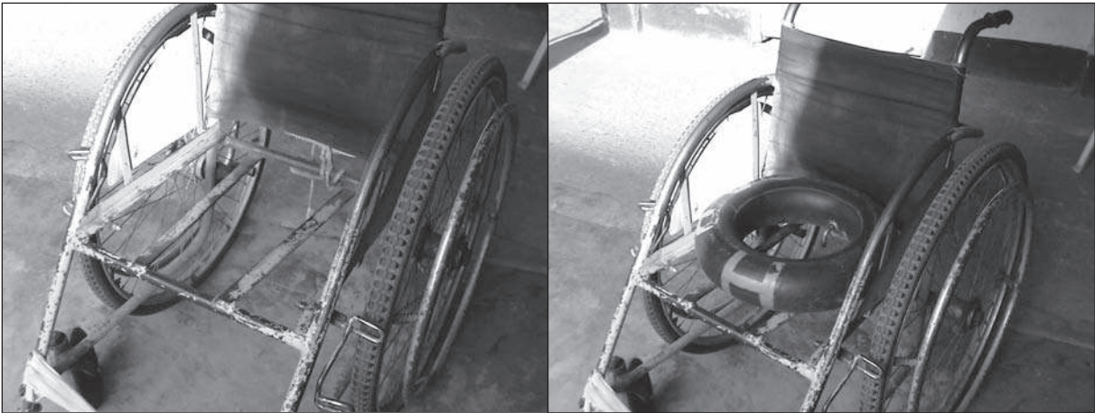
Figures 6.66 and 6.67. Wheelchair convertible to a bathing seat. Wheelchair with cushion and seat board removed and tyre inner tube in place. (Case-study 9.3, page 164)
