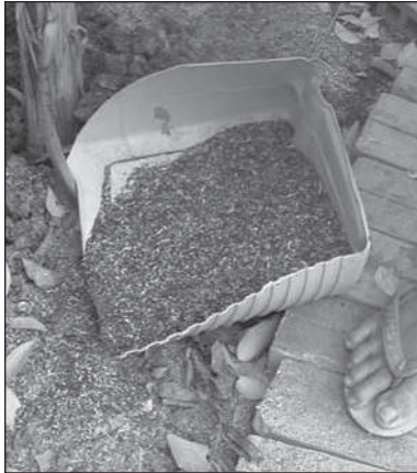
Figure 9.90. Ash scoop made from an old jerry-can.
