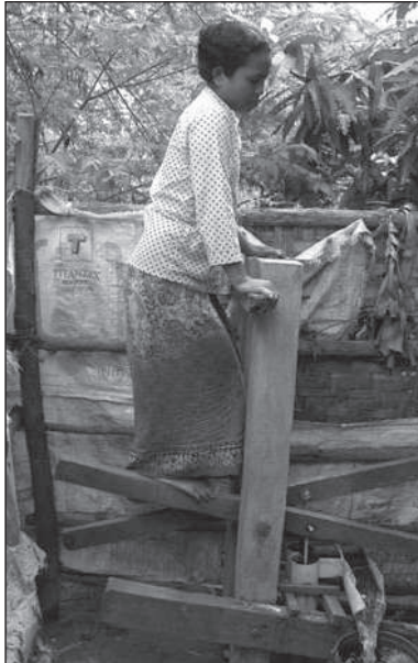
Figure 9.56. Mrs Nourn operates the treadle pump with her feet.
