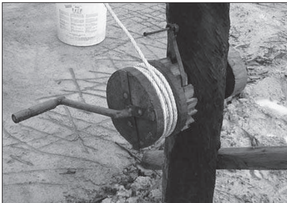
Figure 6.9. Detail of ratchet and pawl winding mechanism. (Case-study 9.11, page 187)
