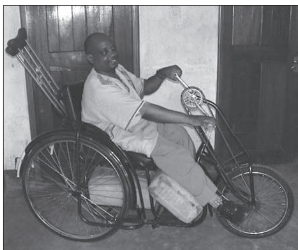
Figure 6.28. Two jerry-cans carried under the seat of this wheelchair. (Case-study 9.24, page 224)
