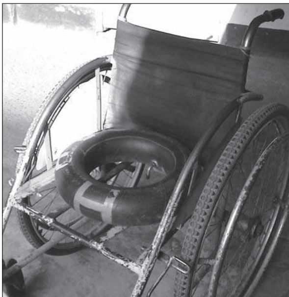
Figure 7.39. Wheelchair with small tyre inner tube in place of seat. Inner tube is durable, easy to clean, widely available at reasonable cost. Suitable for persons with poor sitting balance, so long as it is fully inflated. (Case-study 9.5, page 174)
