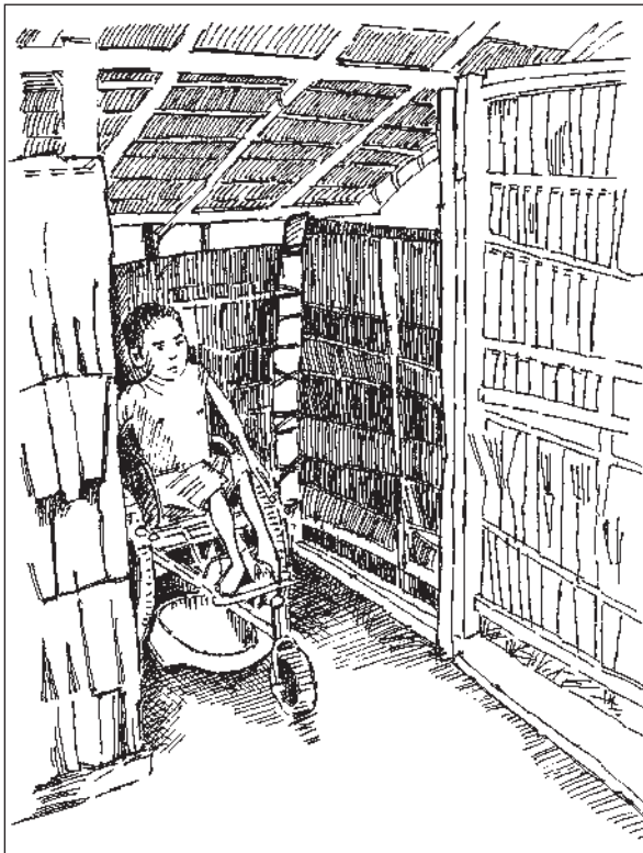
Figure 5.26. Toilet with space to position wheelchair over toilet, but not beside it. The user must reverse in. (Case-study 9.15, page 201)
