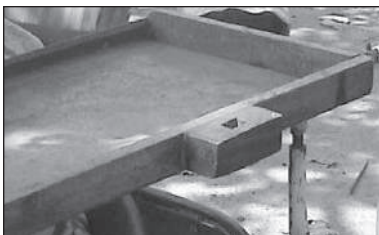
Figure 9.134. The hole in the wheelchair tray to insert the upright post of the implement holder.
